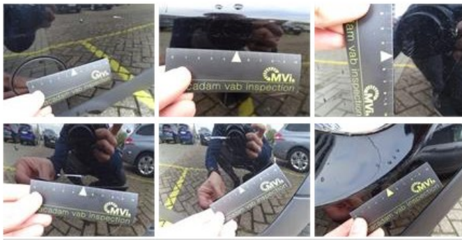
Bonnet, Dent(s) and scratch(es), LI - Repair and paint (complete)
