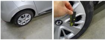
Wheel cover F R, Scratch(es), E - Replace
