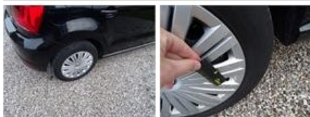
Wheel cover F L, Missing, E - Replace
