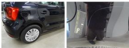
Sill outer R, Deformed / Strained, Le - Replace and paint
