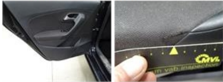
Door F R, Deformed / Strained, Le - Replace and paint
