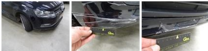
Bumper grille, Broken, E - Replace
