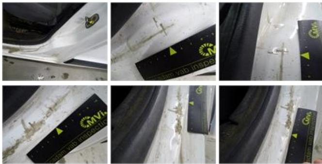
Door frame F L, Dent(s), It - Spot repair
