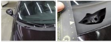
Rearview mirror housing L, Scratch(es), Smart repair
