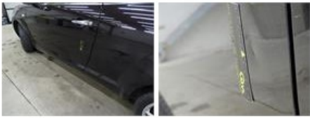
Wing F R, Chemical polution, LI - Repair and paint (complete)
