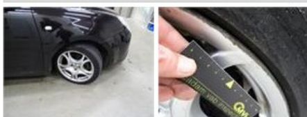
Door F L, Dent(s), PDR - Paintless dent repair
