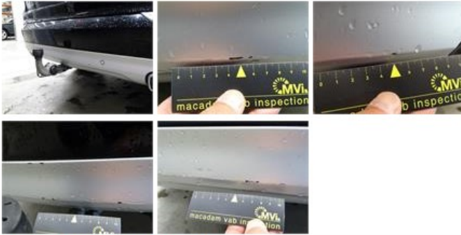
Bumper F R, Scratch(es), It - Spot repair
