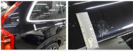
Bumper cover R M, Scratch(es), LI - Repair and paint (complete)
