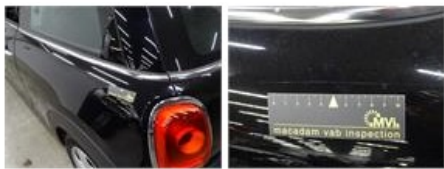
Roof, Dent(s), PDR - Paintless dent repair
