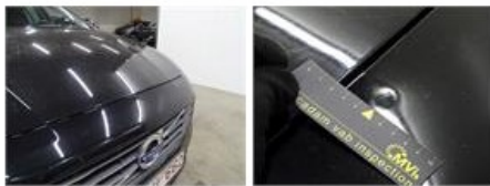
Door frame F L, Scratch(es), It - Spot repair
