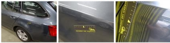
Bumper R, Dent(s), LI - Repair and paint (complete)
