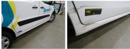
Door R R, Dent(s) and scratch(es), LI - Repair and paint (complete)
