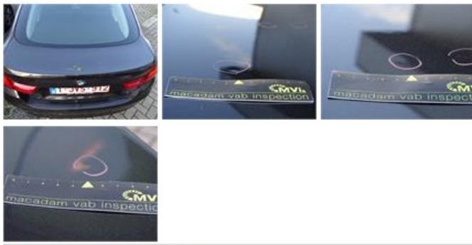
Roof, Hail damage, PDR - Hail
