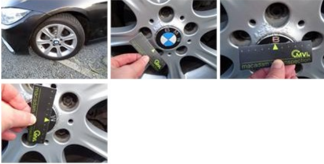
Alloy rim F L, Chemical polution, LI - Repair and paint (complete)
