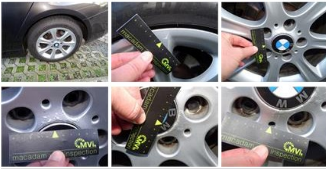
Alloy rim F L, Chemical polution, LI - Repair and paint (complete)
