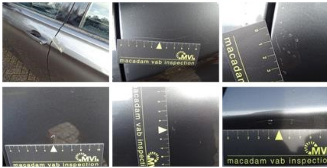
Roof, Scratch(es), LI - Repair and paint (complete)
