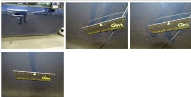
Wing F L, Dent(s), PDR - Paintless dent repair
