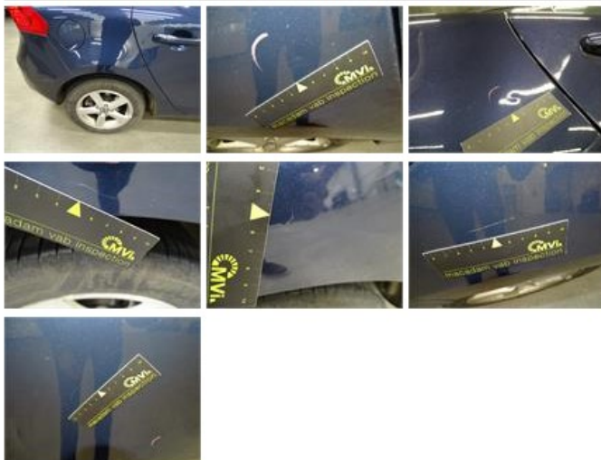
Door F R, Scratch(es), LI - Repair and paint (complete)
