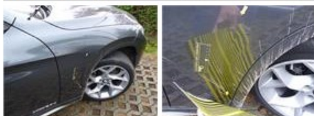
Door trim R R, Deformed / Strained, E - Replace
