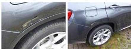
Wing F R, Dent(s) and scratch(es), LI - Repair and paint (partial)
