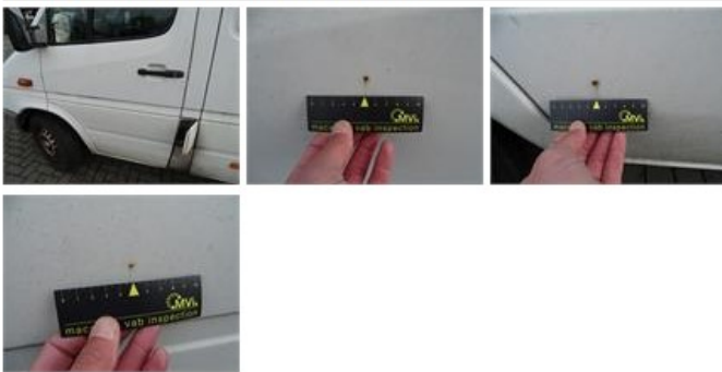
Door F L, Rust, LI - Repair and paint (complete)
