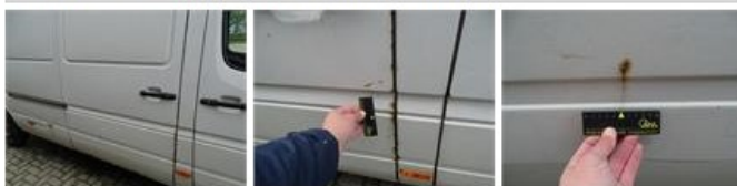
Wing F R, Rust, LI - Repair and paint (complete)
