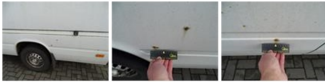
Wing R L, Rust, LI - Repair and paint (complete)
