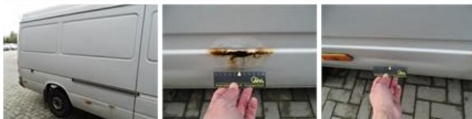
Sidewall RR (LCV), Rust, LI - Repair and paint (complete)
