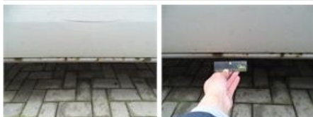
Sidewall RR (LCV), Rust, LI - Repair and paint (complete)
