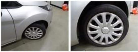
Wing R L, Dent(s), LI - Repair and paint (complete)
