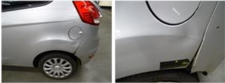
Bumper F, Crack, Le - Replace and paint
