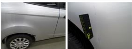
Wing R R, Chemical pollution, LI - Repair and paint (complete)
