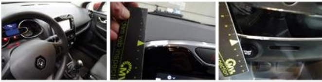
Bumper F, Scratch(es), LI - Repair and paint (complete)
