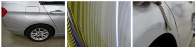
Rocker panel inner F L, Dent(s), LI - Repair and paint (complete)
