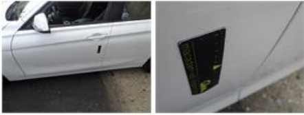
Door panel F L, Scratch(es), Acceptable
