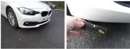
Bumper F R, Scratch(es), It - Spot repair
