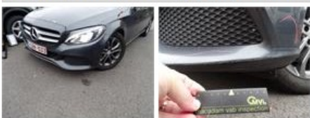
Sill outer R, Dent(s), PDR - Paintless dent repair
