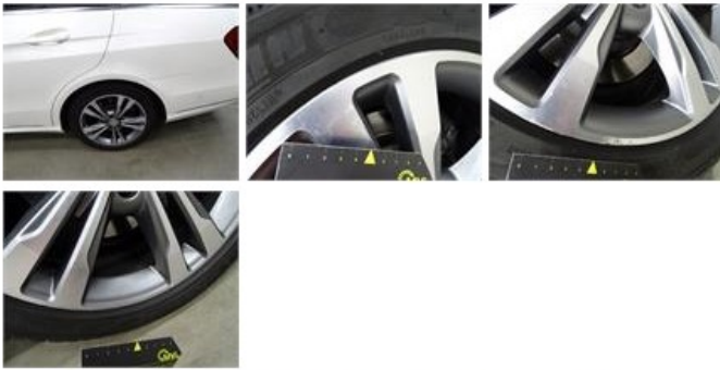
Alloy rim F R polished, Scratch(es), LI - Repair and paint (complete)
