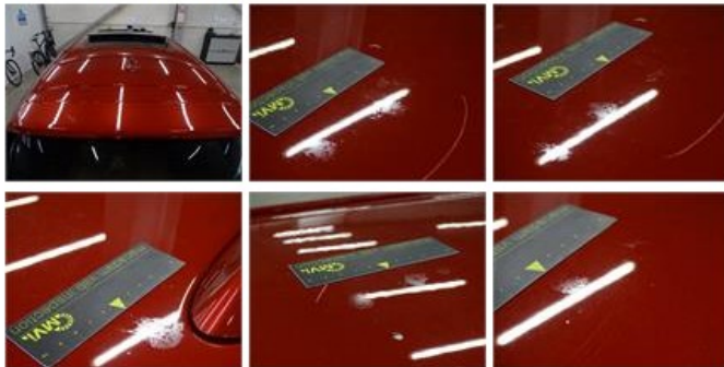
Rear window, Scratch(es), Acceptable
