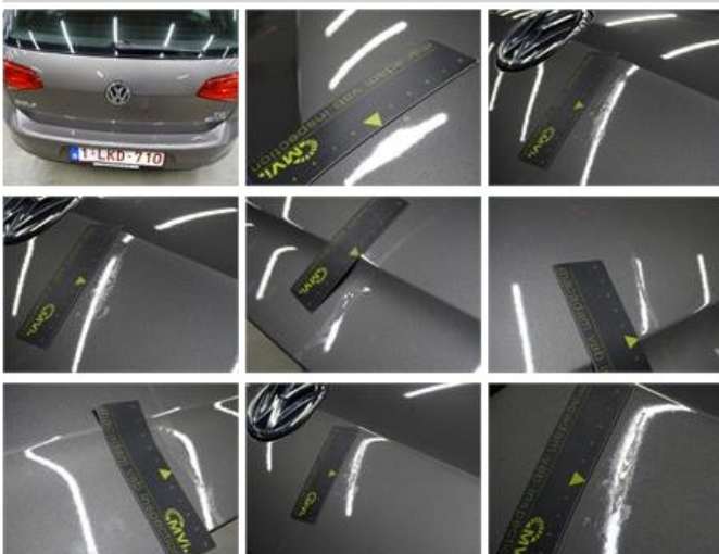
Door R R, Scratch(es), LI - Repair and paint (complete)
