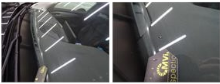
Windscreen, Stone chip(s), Windscreen repair
