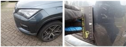
Alloy rim F R polished, Scratch(es), LI - Repair and paint (complete)
