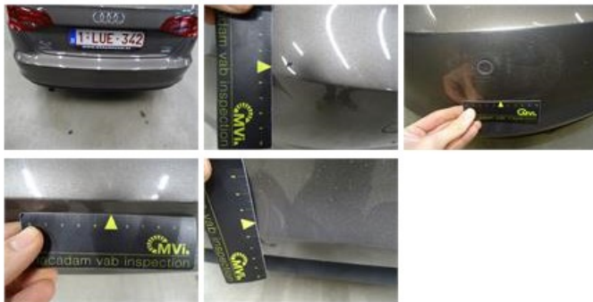
Wing R L, Chemical polution, LI - Repair and paint (complete)
