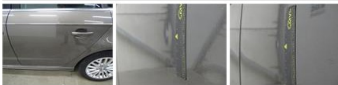
Door R L, Dent(s), PDR - Paintless dent repair
