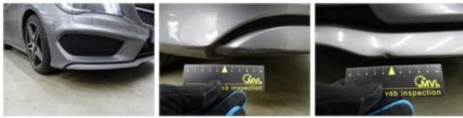
Wheel arch cover F R, Deformed / Strained, E - Replace
