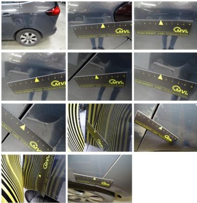
Wing R R, Scratch(es), LI - Repair and paint (complete)
