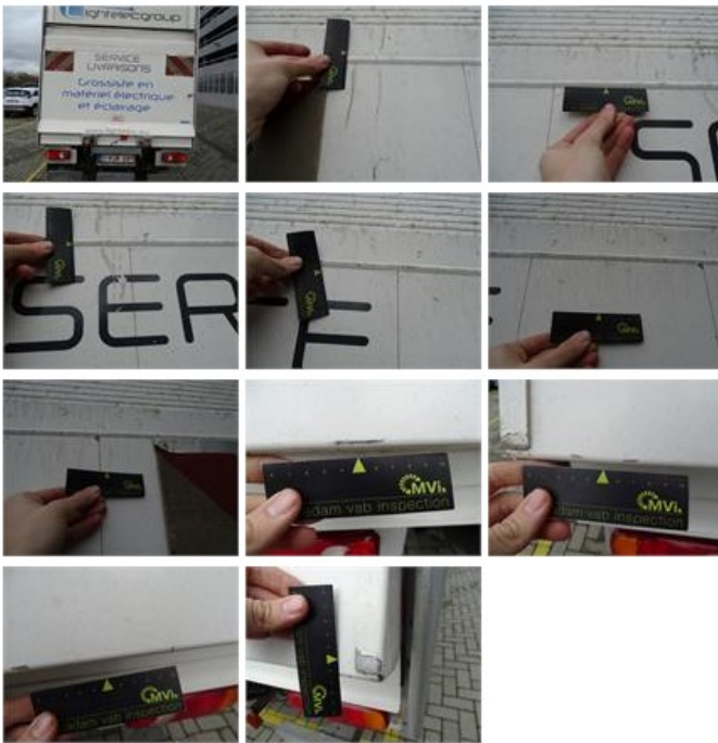
A-Pillar left, Scratch(es), LI - Repair and paint (complete)
