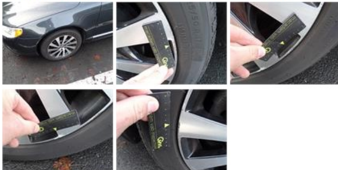
Alloy rim F R polished, Chemical polution, LI - Repair and paint (complete)
