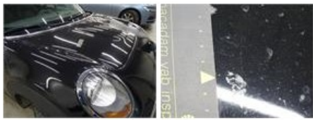
Wing F R, Chemical pollution, It - Spot repair
