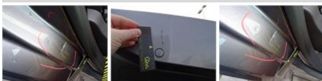
Bumper moulding R, Scratch(es), Smart repair
