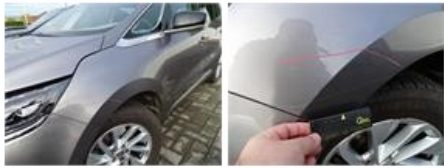
Bumper moulding F R, Scratch(es), E - Replace
