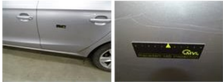
Wing R R, Scratch(es), LI - Repair and paint (complete)
