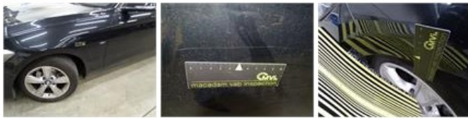
Alloy rim F L, Scratch(es), Acceptable
