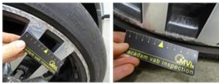
Sill outer R, Scratch(es), LI - Repair and paint (complete)
