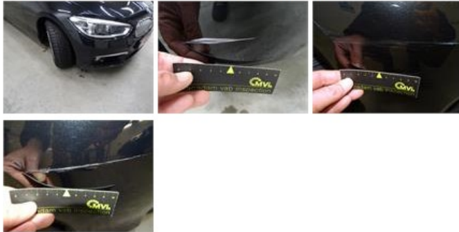
Roof pillar R, Dent(s) and scratch(es), Acceptable
