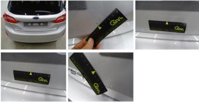
Tailgate, Scratch(es), LI - Repair and paint (complete)
