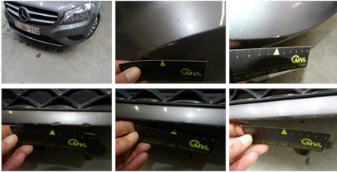
Protection plate M, Deformed / Strained, E - Replace
