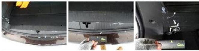
Ceiling, Hole, Smart repair
