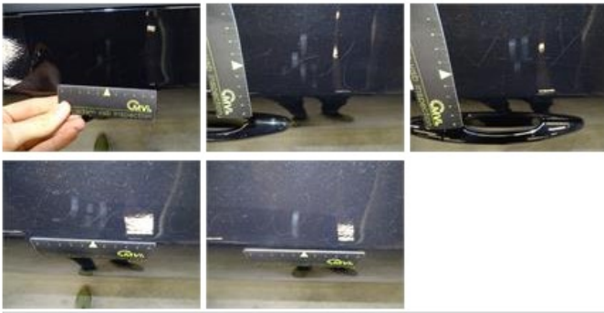
Roof pillar R, Scratch(es), Acceptable
