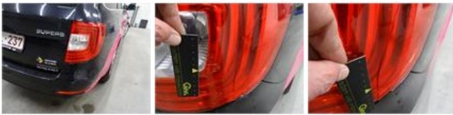
Tailgate, Scratch(es), LI - Repair and paint (complete)
