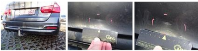
Rocker panel inner R R, Dent(s), LI - Repair and paint (partial)
