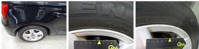
Wing F R, Scratch(es), It - Spot repair
