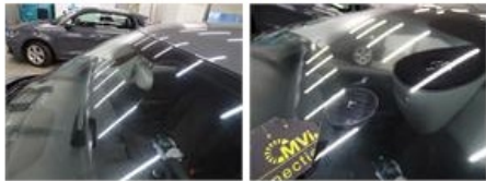
Wing R L, Dent(s) and scratch(es), LI - Repair and paint (complete)
