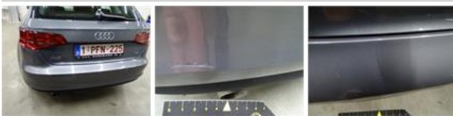
Wing R R, Bad repair, LI - Repair and paint (complete)
