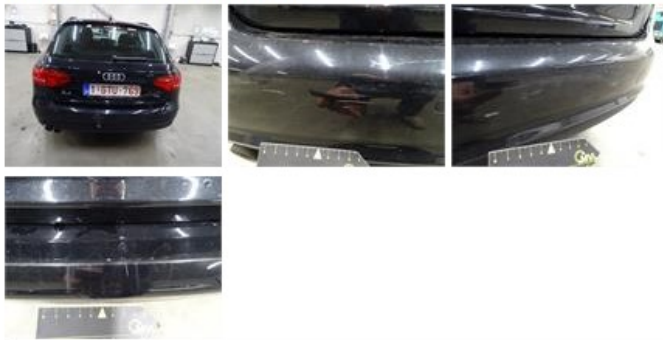
Wing R R, Chemical pollution, LI - Repair and paint (complete)
