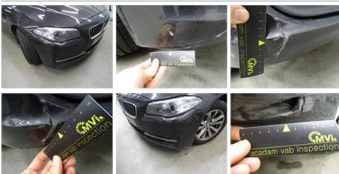
Bumper F, Broken, Le - Replace and paint
