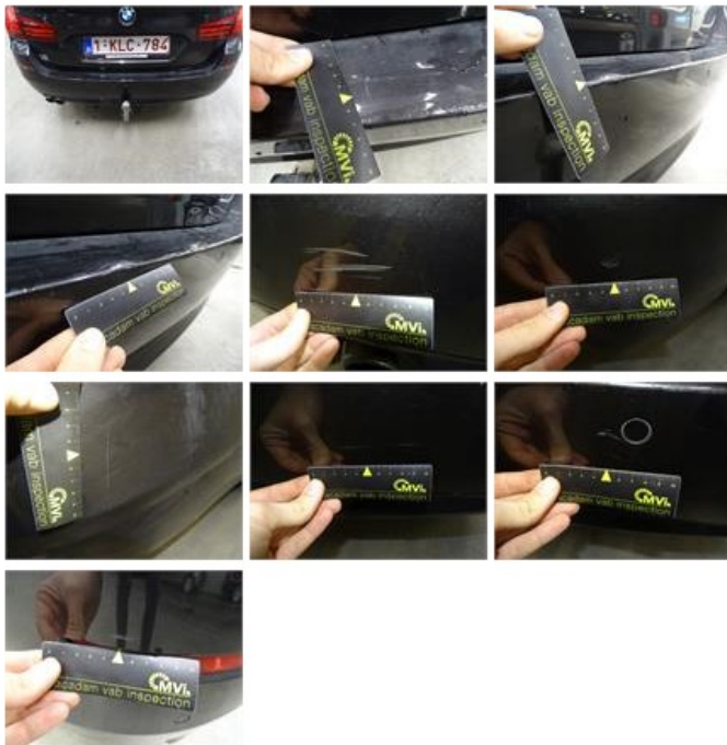
Sill outer L, Dent(s) and scratch(es), Acceptable
