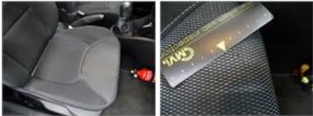
Seat cover F R, Damaged, Acceptable
