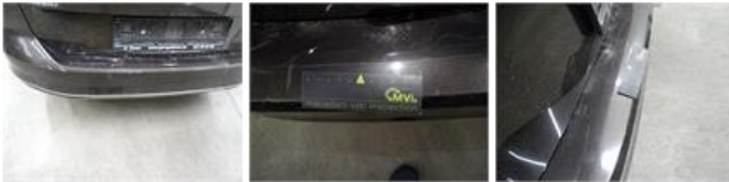
Wing R L, Dent(s) and scratch(es), LI - Repair and paint (complete)
